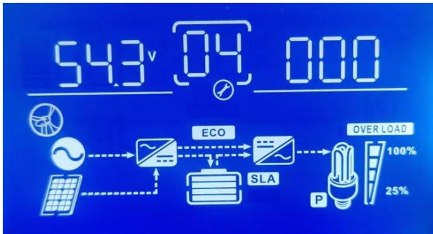
Lead battery float voltage setting display diagram
