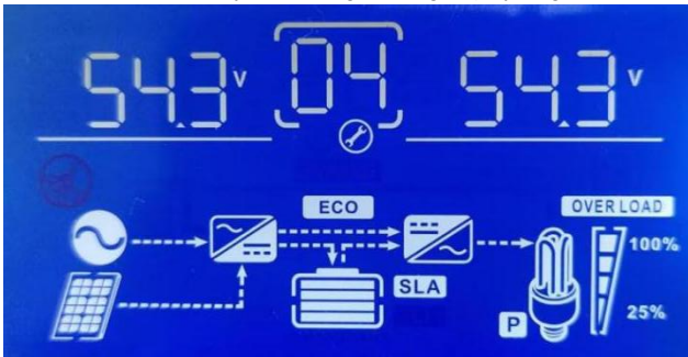
Lead battery float voltage setting successful diagram
