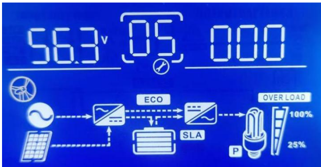
Lead battery average charging voltage setting display diagram
